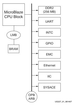
Figure 1: Base System Builder Block Diagram
